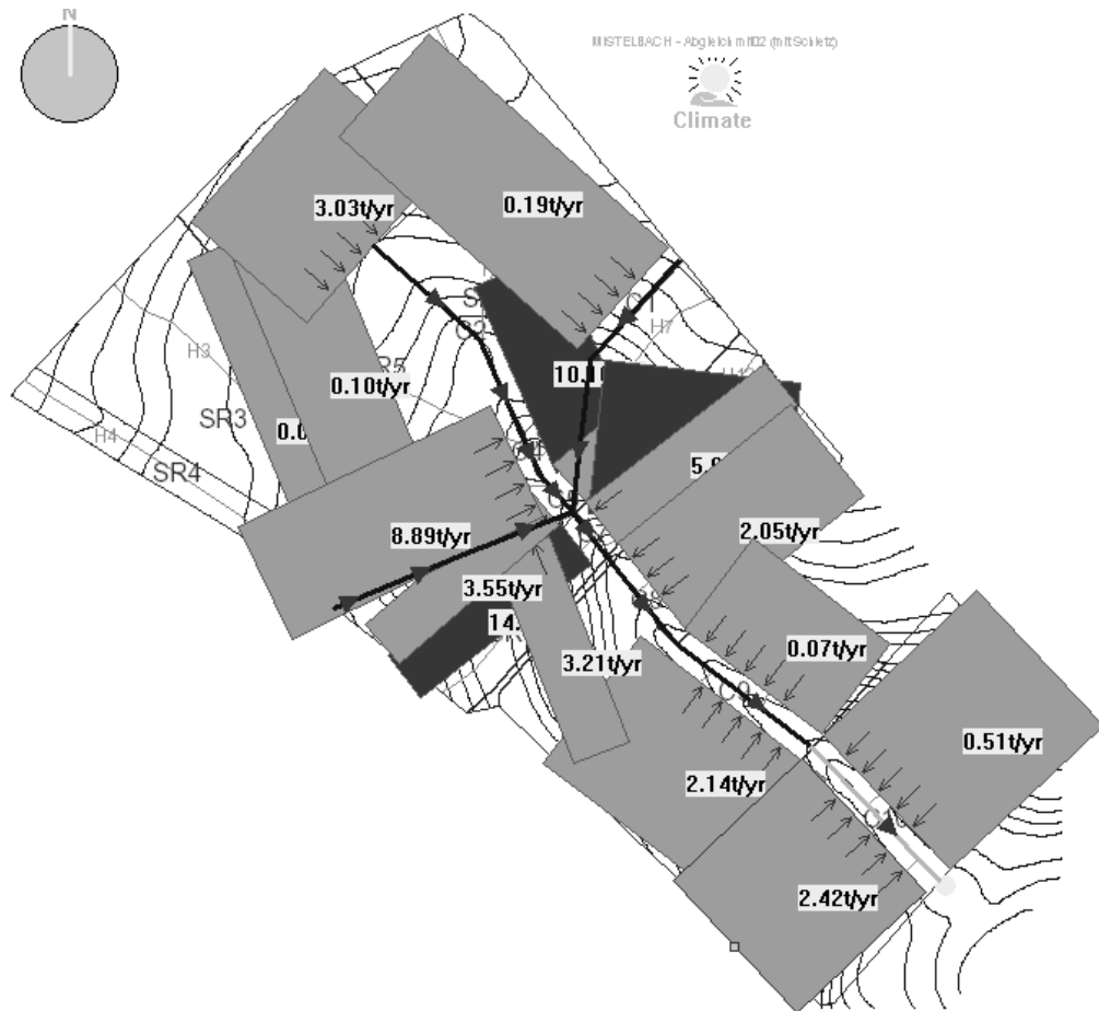
Fig. 5 Sediment delivery from the hillslopes to the channel system within the watershed.
